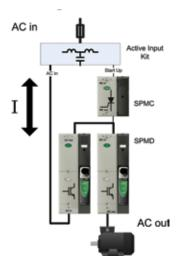
Active inputs for harmonic elimination and regenerating excess energy can be configured with standard drive modules, configured as motoring or regenerating.
